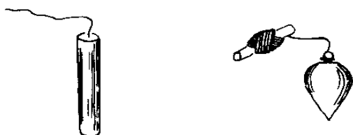
fig 3.2 Plumb bob for vertical marking & leveling
